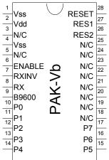
WARNING: The PAK Vb is a static-sensitive, CMOS device. Observe static precautions when handling. Operating the device without both Vss pins grounded or with RES1 or RES2 disconnected may damage the chip.
